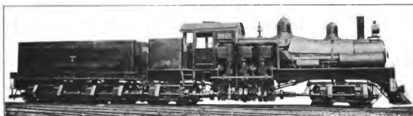
Fig. 131. Sixteen-Wheel Shay Geared Locomotive. Built by the Lima Locomotive & Machine Co. for the Chesapeake & Ohio. Cylinders 3 Vertical 17 in. x 18 in., Working Steam Pressure 200 lbs. per sq. in., Heating Surface 2,332 sq. ft., Diameter of Drivers 46 in., Weight on Drivers 330,000 lbs., Total Weight 370,000 lbs.
